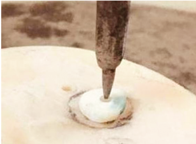
Fig. 5: Pushout bond strength test with UTM using a custom made jig
