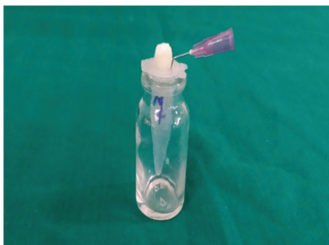
Fig. 1: Experimental model system used to evaluate debris extrusion
